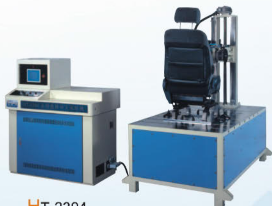
HT-2394 座椅乘降耐久試驗機 Getting In/out Durability Of Seat Cushion Tester
