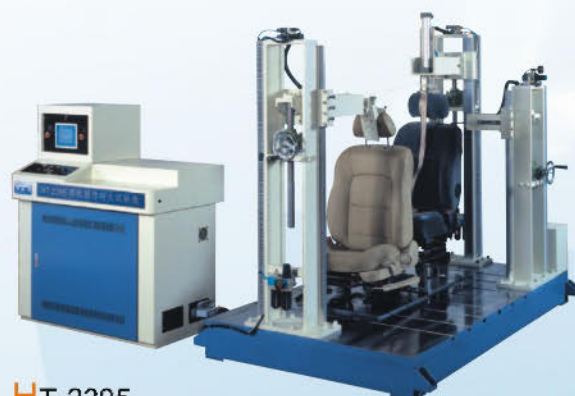
HT-2395 頭枕操作耐久試驗機 Headrest Operation Durability Tester
