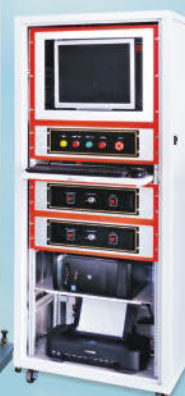
HT-2333B2 動態疲勞試驗機 Dynamic Fatigue Testing Machine
