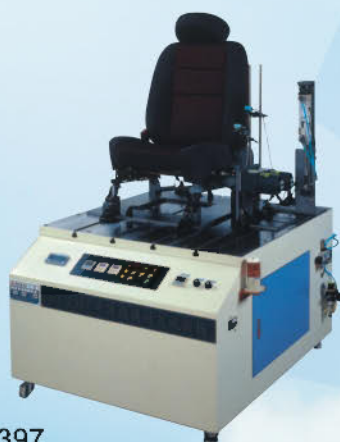
HT-2394 座椅乘降耐久試驗機 Getting In/out Durability Of Seat Cushion Tester
