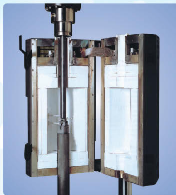
HT-8747 D, E Type High Temperature Chamber
